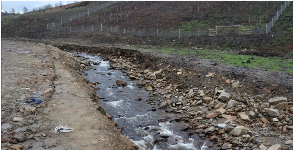
Figure 7: Deposition (right foreground) and erosion (right bank distant) in the recreated Hurst Brook channel.
